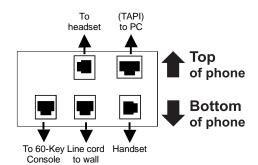
Connectors on bottom of 48-Key Digital Feature Phone (headset jack shown)
