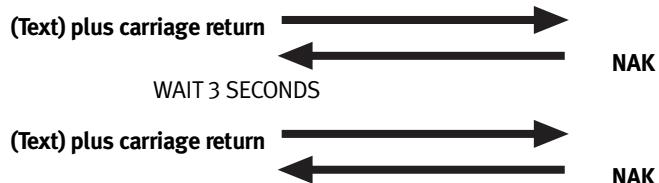
PMS responds, but cannot accept data at this time. PhoneBill will re-transmit data after 3 seconds until the PMS accepts the message, or until 2 NAK responses are received, at which time the PMS data message is dumped to the printer.
