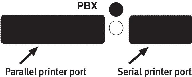
If the PBX LED does not flicker, confirm that TD of the PBX (usually Pin 2 [Mitel Pin 3]) is connected to Pin 3 of PhoneBill and that the PBX signal ground (usually Pin 7) is connected to Pin 7 of PhoneBill. Additionally, if the PBX requires hand-shaking, consult the PBX manual.
