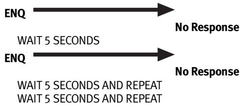
PhoneBill will re-transmit an ENQ every 5 seconds until the PMS accepts the message, or until 4 successful ENQ responses have been sent, at which time the PMS data message is dumped to the printer.
