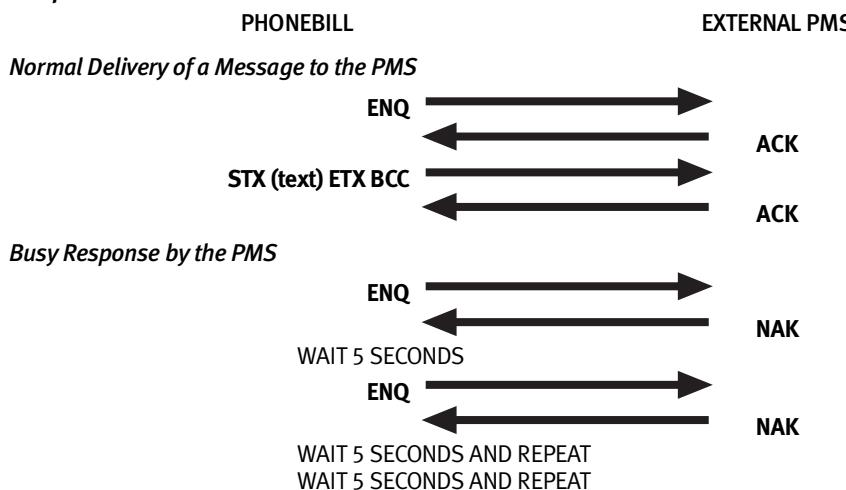
PMS responds, but cannot accept data at this time. PhoneBill re-transmits an ENQ after 5 seconds until the PMS accepts the message, or until 4 NAK responses are received, at which time the PMS data message will be dumped to the printer.
