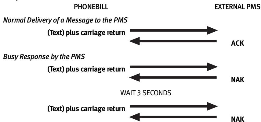
PMS responds, but cannot accept data at this time. PhoneBill re-transmits data after 3 seconds, or until 2 NAK responses are received, at which time the PMS data message will be dumped to the printer.
