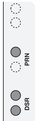
**Top DSR LED illuminated** — Indicates wrong polarity on DTR of printer. Verify Pin 4 is connected to the printer DTR (usually Pin 20) and that the printer is programmed to perform hardware handshaking at the DTR Pin and the proper polarity is set.
