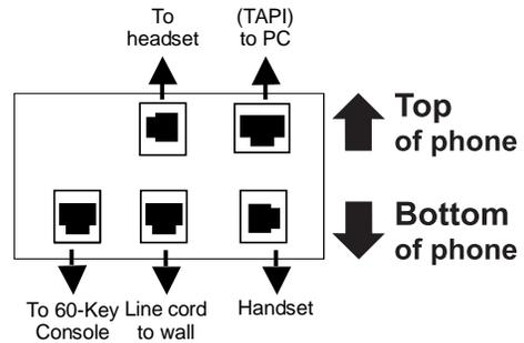
*Connectors on bottom of 48-Key Digital Feature Phone; TAPI model shown (headset jack is **only** on 48-Key Feature Phones shipped after March 1, 2004)*
